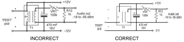
**The Incorrect Circuit:** The wiring for the primary of T1 is wrong.
